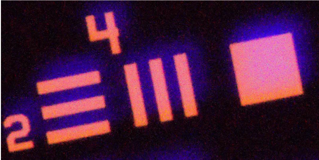
Figure 60 – Resolution target imaged with all RGB color with a sign of lateral chromatic aberration for blue. The blue image is shifted to up-right direction.
